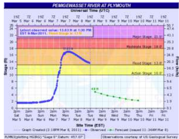
Stream gauge at bridge indicating change in river level in early March 2011.
